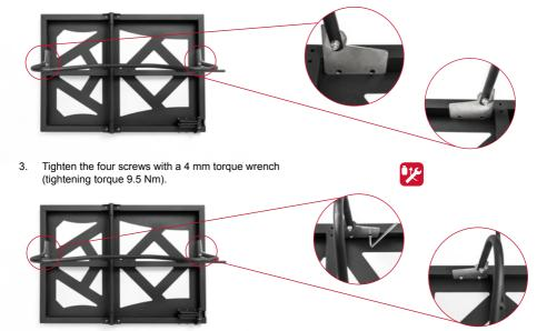
Hook the springs in the holes in the middle of the stand and the base plate. 4.
