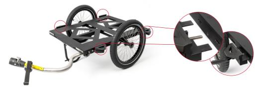
To attach the aluminum box, loosen the clamping jaws slightly so that the railing of the box slips between the base frame and the clamping jaws when this is put on. Then screw the clamping jaws tight and turn the quick release.
